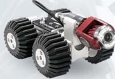
ROVVER 125 chassis with sediment wheels, raise kit and zooming pan/tilt camera.
