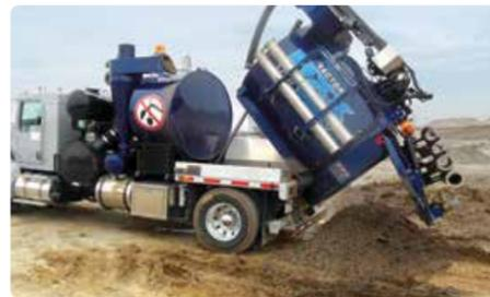
The vacuum system features ultra-efficient airflow, a Vactor trademark. The simplified airflow path maximizes pickup and filtration effectiveness, while minimizing the amount of material that passes through the blower. This, in turn, reduces the likelihood of premature wear or extensive repairs.
